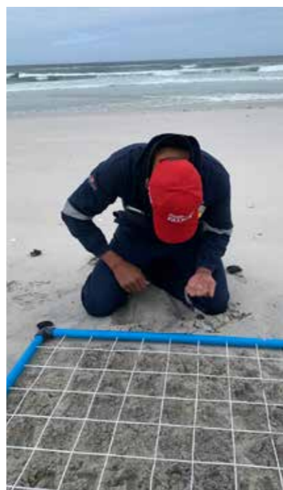
FIGURE 14B Examples of semi-quantitative and quantitative survey methods for determining levels of plastic pellet shoreline contamination
