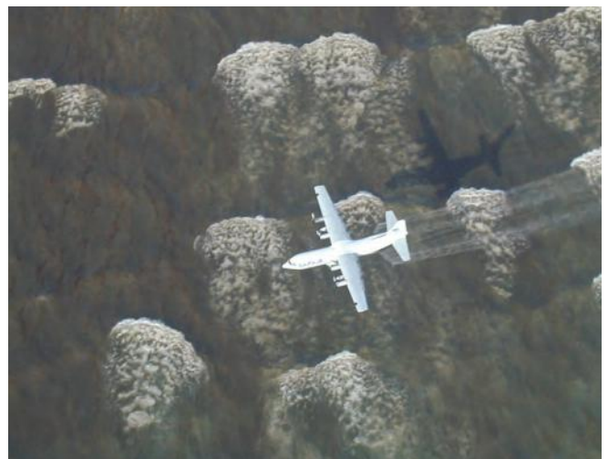
▲ Figure 10: Application of dispersant from a multi-engine aircraft. Here, application in shallow waters was considered beneficial.
