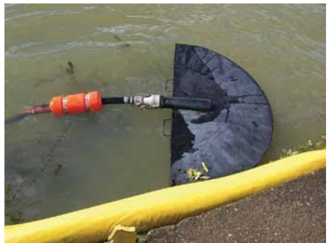
▲ Figure 11: Fixed weir skimmer attached to a vacuum pump. A number of small inlets at the edge of the head allow oil to be selectively recovered. For use in calm water with minimal debris (Image courtesy Lamor).
