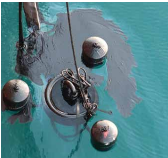
▲ Figure 10: Workers placing a hose attached to a vacuum pump directly into the oil. In this instance, the small weir attachment has been removed to allow the viscous fuel oil to flow into the hose, with a consequent potential increase in entrained water.
