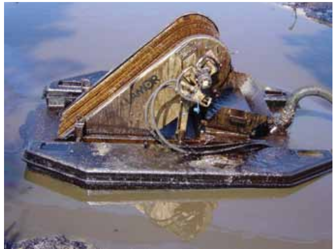
▲ Figure 5: Free floating brush skimmer. Oil adheres to the rotating brush sets and is lifted from the water surface. A comb removes the oil from the brushes to storage. A propeller behind the brush draws floating oil towards the skimmer to enhance the encounter rate and throughput (Image courtesy Lamor).
