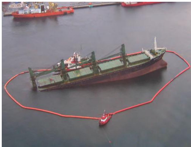
▲ Figure 12: Inflatable boom moored around a partially sunken wreck to contain any potential leakage of bunker fuel.
