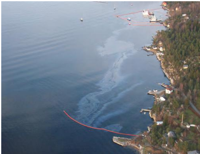
▲ Figure 14: Boom used as a spur to deflect oil to the shore for recovery (© Norwegian Coastal Administration).
