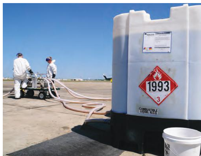
▲ Figure 12: Use of 1m 3 Intermediate Bulk Containers (IBCs) allows straightforward storage and handling of dispersant. (Image courtesy USCG).
