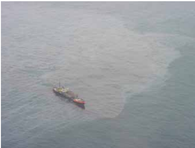
▲ Figure 18: A recovery vessel in a large and homogeneous slick of thick oil, allowing highly effective use of resources.
