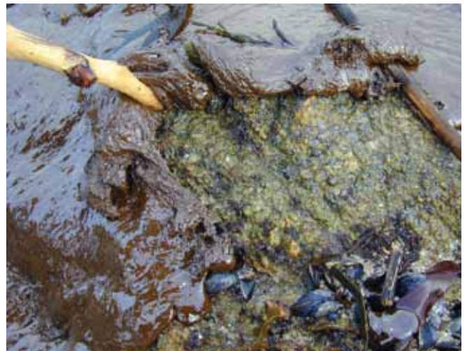
▲ Figure 5: Close-up image of emulsified heavy fuel oil, showing the highly viscous consistency. The high levels of water in the oil reduce the ability of the oil to adhere to underlying substrate.
