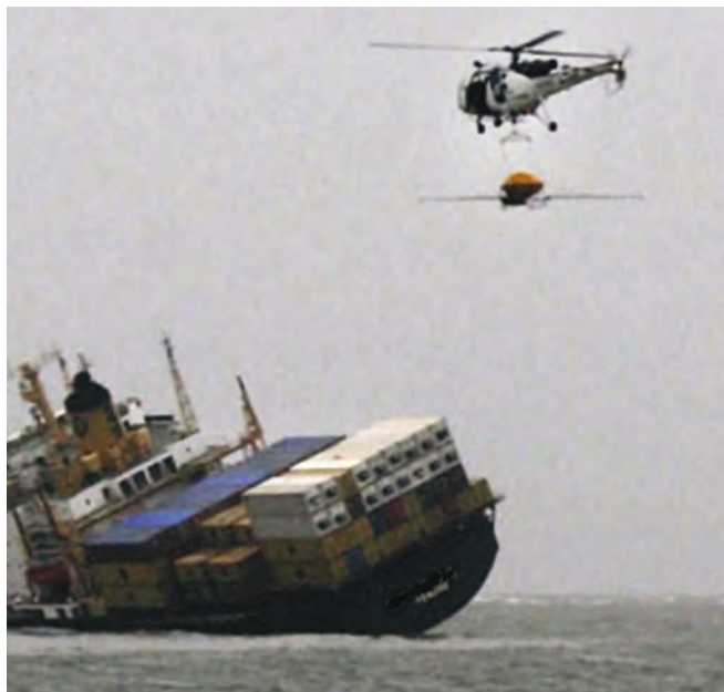
▲ Figure 11: A helicopter, with an under-slung spray system, approaching a fresh spill of fuel oil. To be effective, application from a lower altitude would be necessary. (Image courtesy of Indian Coastguard).
