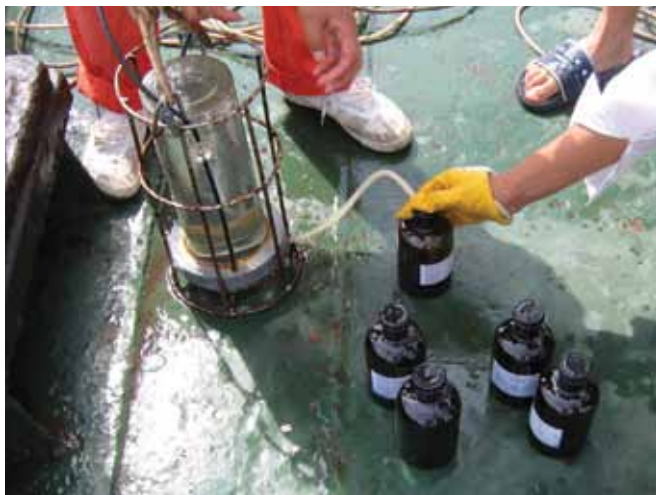
▲ Figure 8: Decanting water samples from the sample collection device into glass bottles, for split samples.
