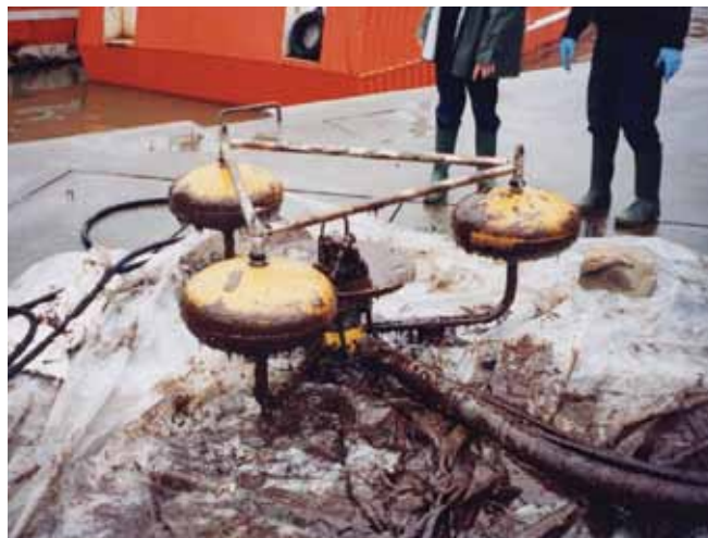
▲ Figure 37: A weir skimmer brought ashore after recovery of heavy oil. Following demobilisation, equipment should be cleaned and overhauled in readiness for future use.
