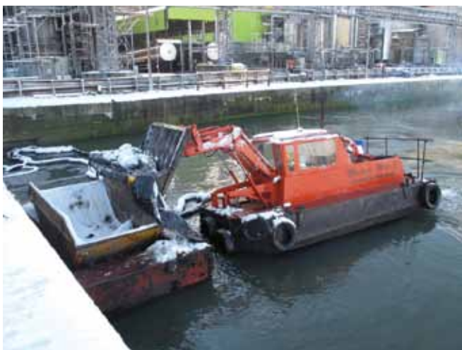
▲ Figure 35: Self-propelled vessel, normally used to recover debris in a port. Here, the low temperature and relatively high pour point of the oil caused the oil to become semi-solid, necessitating recovery by scoops and grabs into a floating skip.
