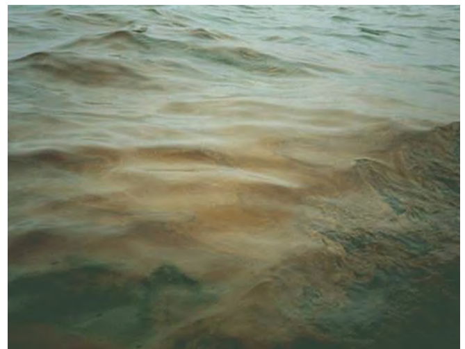
▲ Figure 6: Dispersion starting after application to Forties Crude during the SEA EMPRESS spill. (Image courtesy of AEA Technology).
