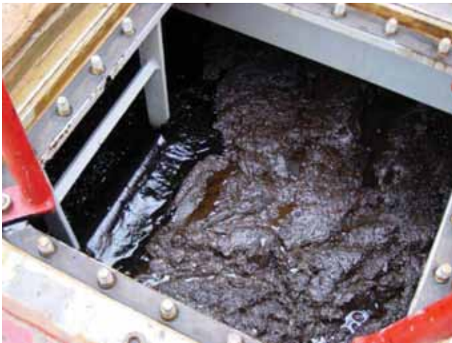
▲ Figure 25: Highly viscous recovered oil in a storage tank on board a recovery vessel (Image courtesy NOFO).
