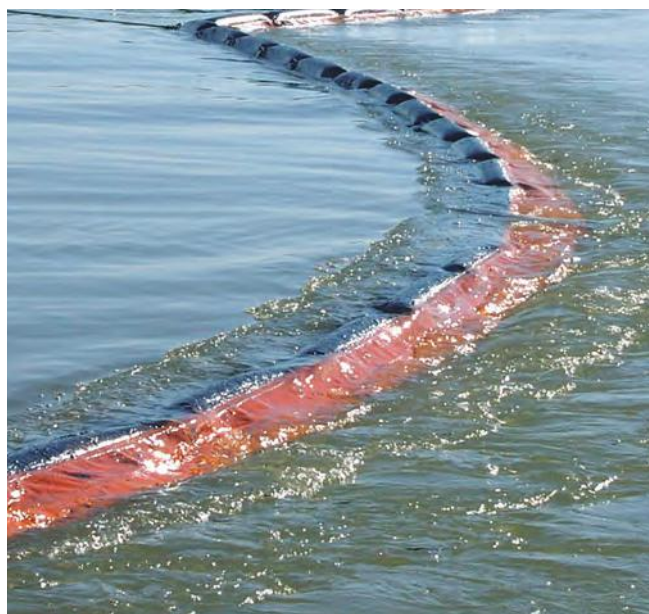
▲ Figure 4: The strong current has caused the boom to plane, allowing any oil to be lost under the skirt.
