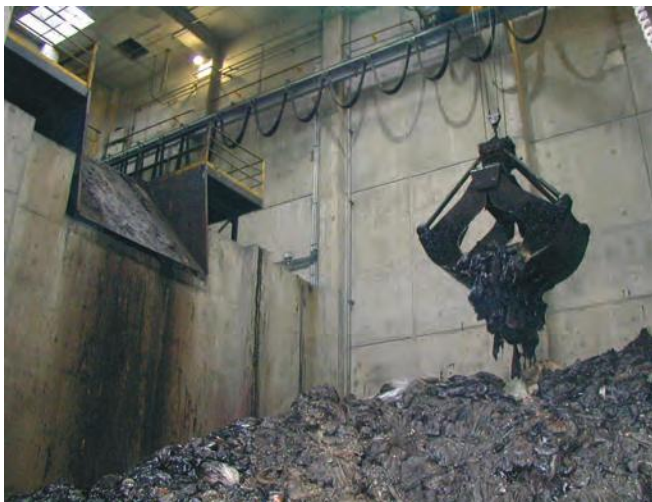
▲ Figure 19: Sacks of oiled waste being fed into the loading chute of a large industrial incinerator for co-disposal with domestic waste.
