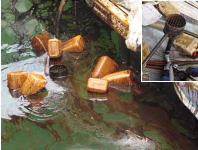
▲ Figure 14: Improvised weir skimmer constructed from plastic bottles and metal offcuts, attached to a vacuum pump. This device allows rudimentary recovery and can be adjusted by removal or addition of bottles.
