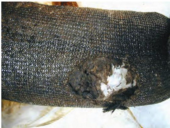
▲ Figure 4: The surface of a continuous, homogeneous sorbent boom cut away to show only partial use. The inner volume remains unsoaked, either because the boom has been deployed for an insufficient period or because the oil is too viscous to penetrate into the structure.
