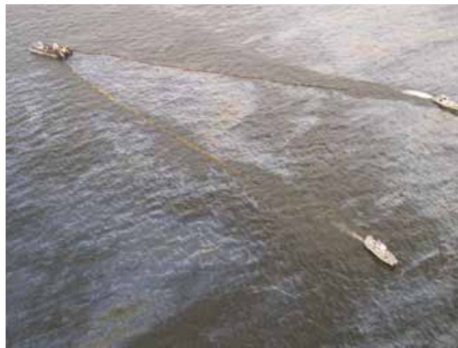
▲ Figure 30: A belt skimming vessel deployed with boom and towing vessels in a V configuration.
