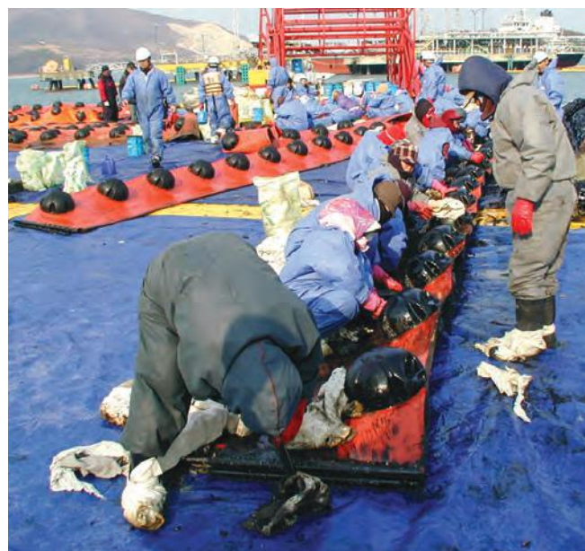
▲ Figure 6: Oil trapped behind external floats of fence boom can be particularly difficult to clean.
