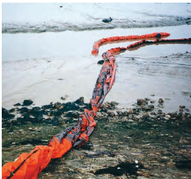
▲ Figure 5: A boom can be easily damaged once deployed. Regular attention is required to ensure its effectiveness is maintained throughout the tidal cycle.
