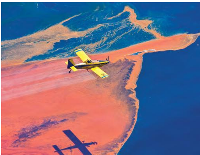
▲ Figure 9: An Air Tractor spraying from an under-wing spray boom onto crude oil spill from an offshore platform. (Image courtesy of Mark Hamilton Photography).
