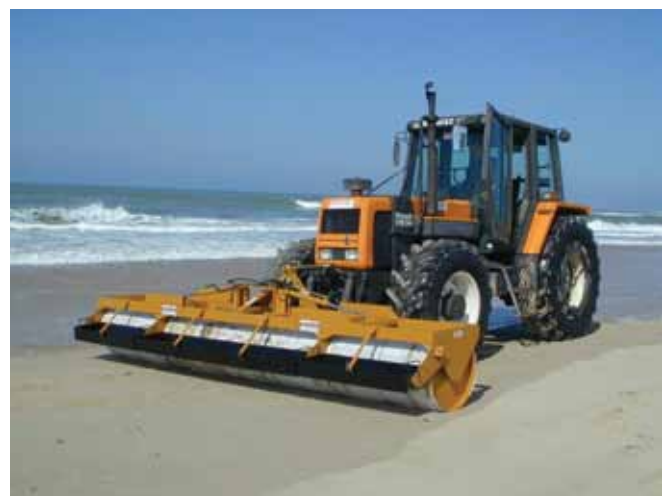
▲ Figure 36: Tractor-mounted oleophilic drum skimmer, used to collect fresh tarballs on a hard-packed sand beach (Image courtesy Le Floch Dépollution).
