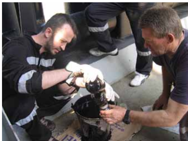
▲ Figure 4: Decanting a bunker fuel source oil sample on board a casualty.
