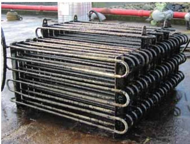
▲ Figure 27: Portable heating coil used to assist with discharge of viscous oil from recovery vessels to shore.
