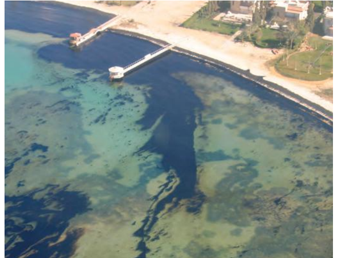
▲ Figure 15: Heavy fuel oil arriving at the shoreline. Benthic seagrass and seabed rock formations can confuse estimations of the amount of oil.
