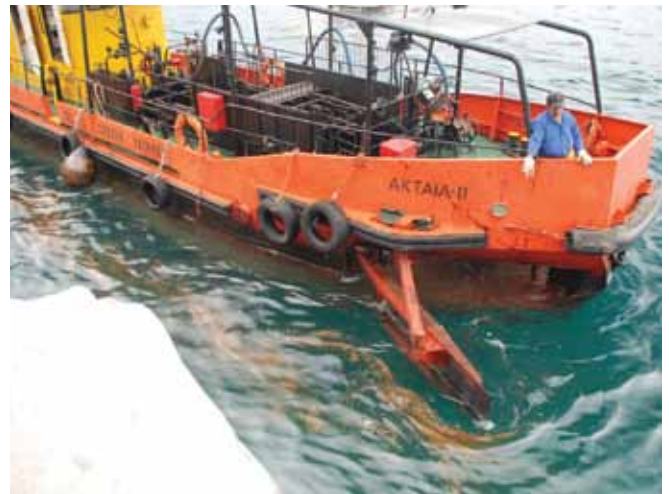
▲ Figure 1: A self-propelled weir skimmer for use in ports and nearshore waters. The bow doors open to enhance the swath and allow entry of floating oil. Recovered oil is pumped to an internal storage tank.
