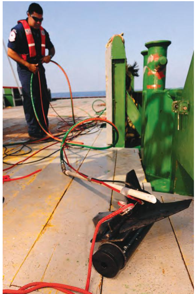
▲ Figure 13: Preparing a towed fluorimeter to measure dispersant effectiveness at sea. (Image courtesy USCG).
