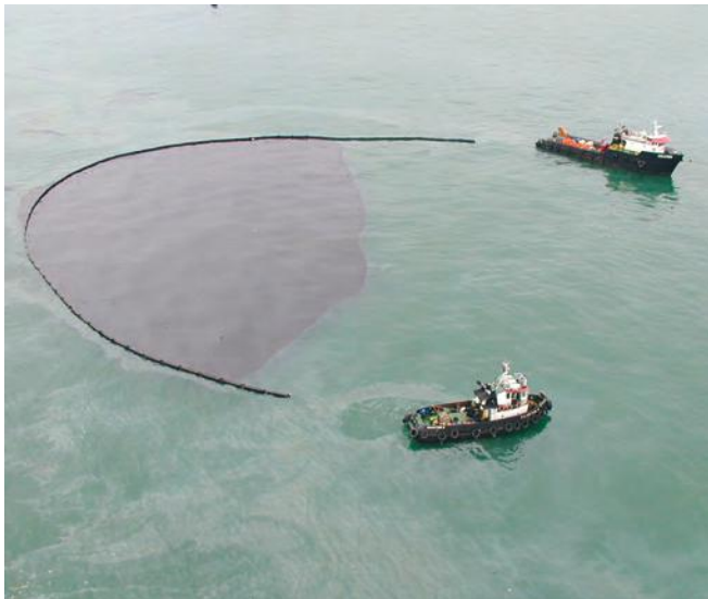
▲ Figure 8: Inflatable boom deployed in a U configuration between two vessels to contain a heavy crude oil. Recovery of the oil will bring the operation to a successful conclusion.
