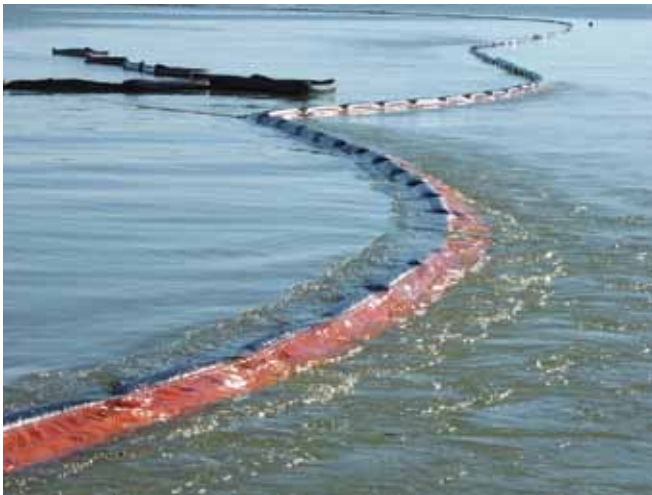
▲ Figure 4: Full awareness of the limitation of equipment and of the environments into which they are deployed will help to ensure time and effort is not wasted on actions that can be foreseen not to work. Here, high currents mean the boom will be unable to contain oil.
