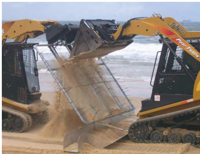
▲ Figure 17: Mechanical sieving of tarballs from sand in order to reduce the amount of waste generated.
