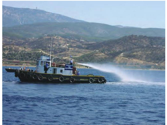
▲ Figure 8: Application of dispersant using fire monitors on a tug, showing uneven spread of dispersant and the effect of wind.
