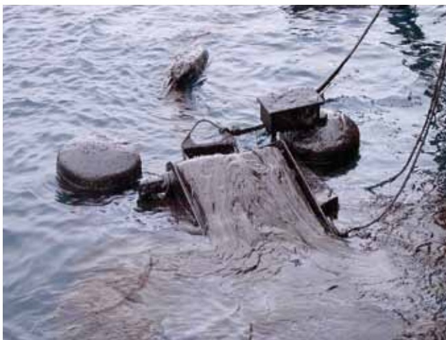
▲ Figure 16: A belt adaptor added to enhance the capability of the base weir skimmer in highly emulsified fuel oil. The high viscosity of the oil prevented its flow towards and over the lip of the weir. Instead, the toothed belt adaptor 'grabbed' the oil enhancing the efficiency, with the cohesive energy of the oil causing the remaining oil to 'flow' toward the skimmer (Image courtesy Ro-Clean Desmi/Danish Navy).
