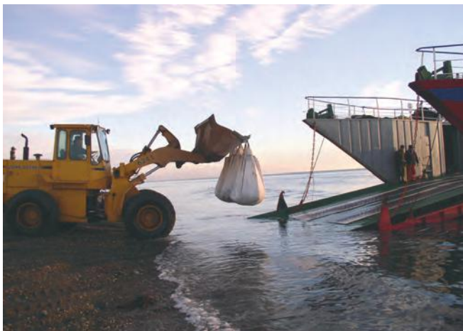
▲ Figure 11: Smaller bags of oiled waste consolidated into one tonne 'big-bags' are transported onto a landing craft for removal from an isolated shoreline.
