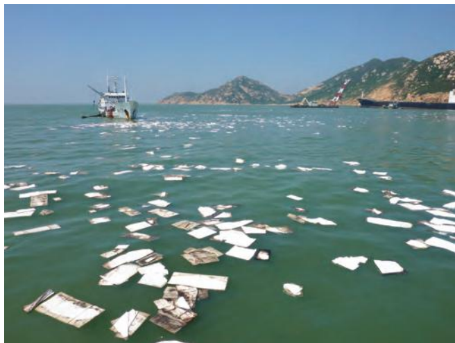
▲ Figure 11: Sorbent pads applied at sea. Considerable effort will be required to subsequently recover the pads to eliminate secondary contamination. Use of containment boom and skimmers may afford a more effective means of recovering the oil than the use of sorbents.
