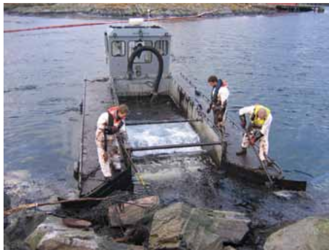
▲ Figure 34: Self-propelled weir skimmer recovering oil at a sheltered rocky inlet. The shallow draft of the vessel allows work close to shore. Operators assist by moving oil towards the mouth of the weir.
