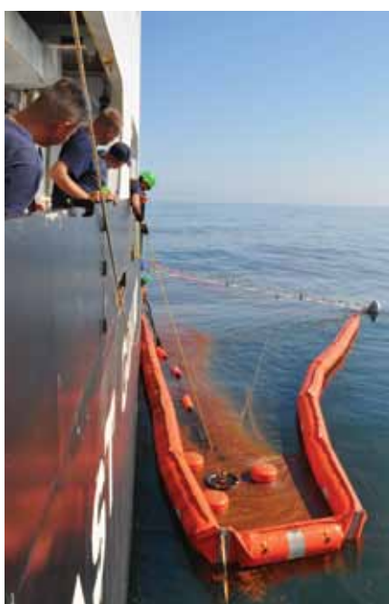
▲ Figure 29: Boom towed in a U configuration with a skimmer deployed from the main recovery vessel.
