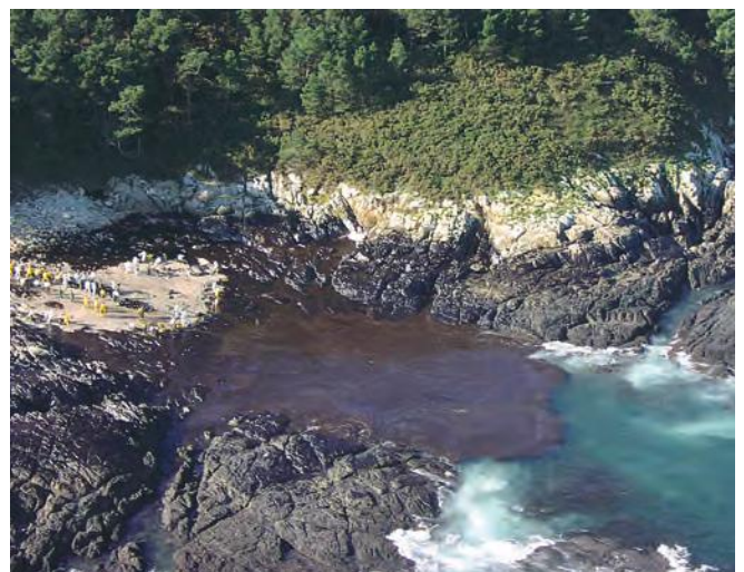
▲ Figure 19: Emulsified heavy fuel oil held against the shore by wind and waves. The thickness of the oil is difficult to estimate as the extent to which the oil is pooling in crevasses between the rocks cannot be readily determined from the air.
