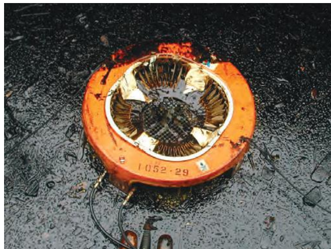
▲ Figure 15: Disc skimmer working successfully in a freshly spilled light crude oil. However, were the oil to become significantly emulsified, the effectiveness of the recovery operation would reduce due to the inability of the emulsion to adhere to the discs.
