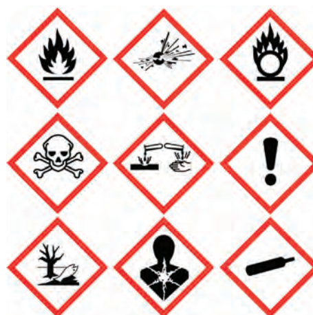
▲ Figure 7: GHS pictograms for HNS labelling. Left to right: flammable, explosive, oxidising, acute toxicity, corrosive, harmful/irritant, toxic to the environment, carcinogen/sensitiser and compressed gas. These are intended to replace national and regional labels.
