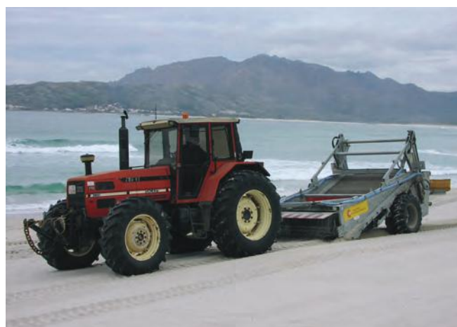
▲ Figure 26: A tractor-towed beach cleaning machine collecting tarballs.
