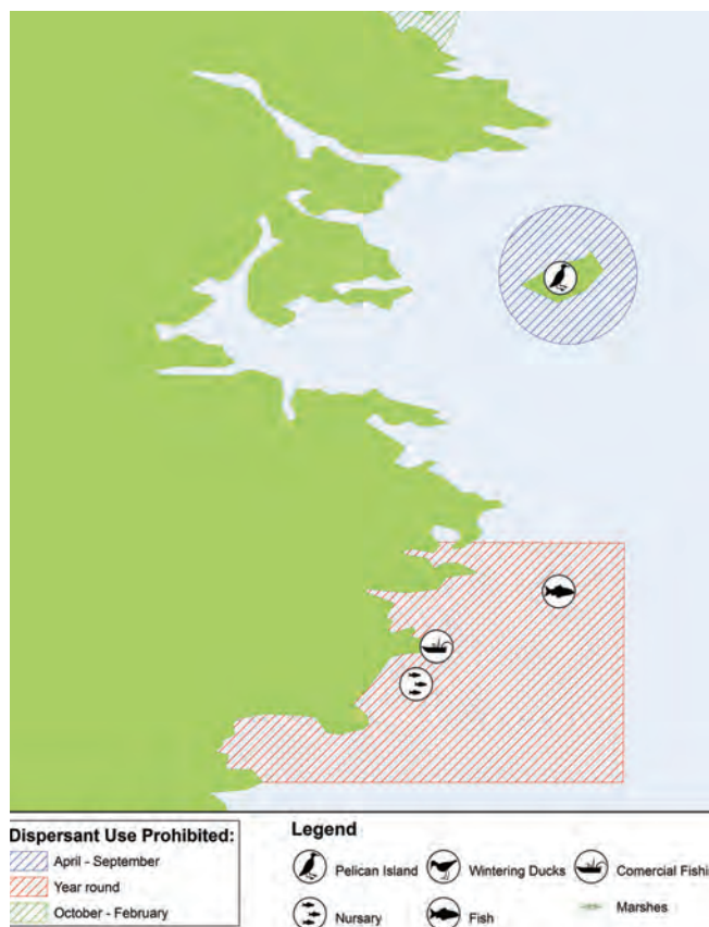
▲ Figure 17: Sensitivity maps are often used in contingency plans to delineate where and when dispersants can be used. In the example, dispersant use is prohibited in the red area because of year-round commercial fishing, but is pre-approved seasonally for treating oil around a bird colony at Pelican Island (blue). Use in shallow water, close to the mainland may be allowed in special circumstances, for example to protect the mangroves or marsh which are both highly sensitive to stranded oil.
