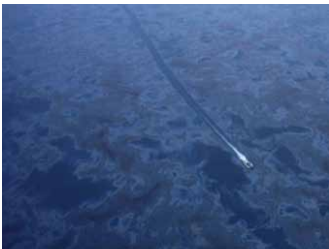
▲ Figure 19: As the oil spreads and starts to fragment, the encounter rate decreases, necessitating greater effort to recover.
