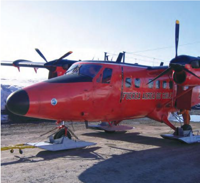
▲ Figure 2: Twin engine fixed-wing aircraft with high wings are ideal platforms for aerial observation of oil at sea. Helicopters may be preferable for observation closer to shore due to their greater manoeuvrability and slower speeds.
