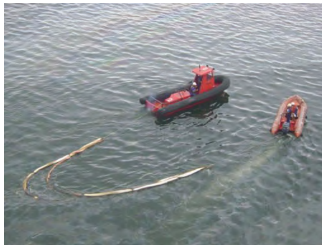
▲ Figure 12: Sorbent boom towed in a 'U' formation behind two vessels, with the aim of recovering sheen (very thin oil films) at sea. Saturation of the boom by seawater limits its effectiveness and the lack of skirt on the boom limits the ability to contain oil. Here oil can be seen escaping from the boom.
