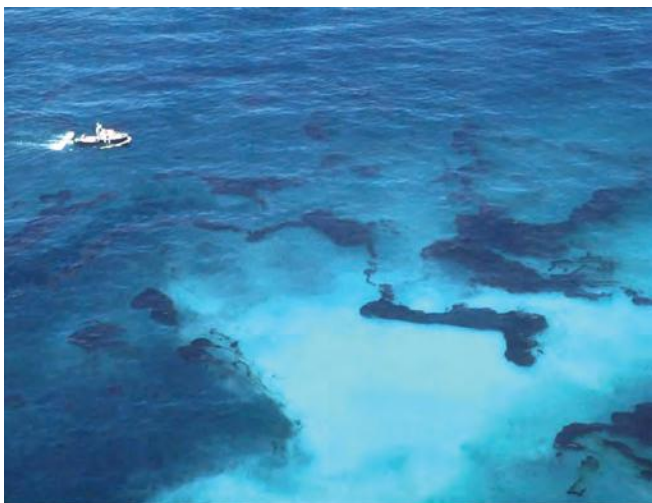
▲ Figure 5: Ineffective treatment of a heavy fuel oil with dispersant is characterised by a white plume in the water. The oil remains unaffected.
