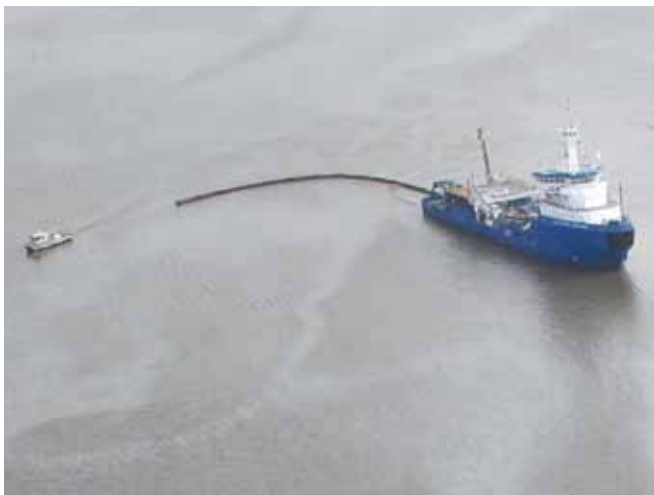
▲ Figure 29: Boom towed in a U configuration with a skimmer deployed from the main recovery vessel.
