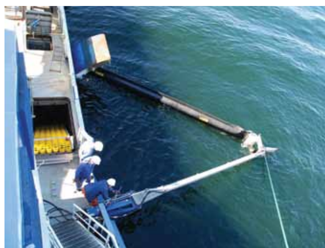
▲ Figure 32: An in-built single ship recovery system. Boom stored in a compartment at the side of the vessel is deployed through an opening by an on-board crane. The opening also allows entrained oil to be recovered by the in-board skimmer, here comprising six sets of brushes in a conveyor arrangement (Image courtesy Lamor).
