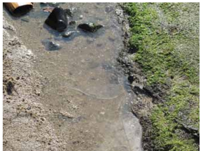
▲ Figure 7: A translucent base oil, used in the manufacture of lubricating oils, has formed lenses on the water surface. This oil was difficult to quantify due to its lack of colour.
