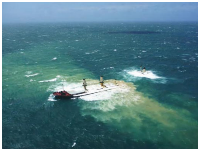
▲ Figure 17: Plume of rock phosphate escaping from a casualty.
